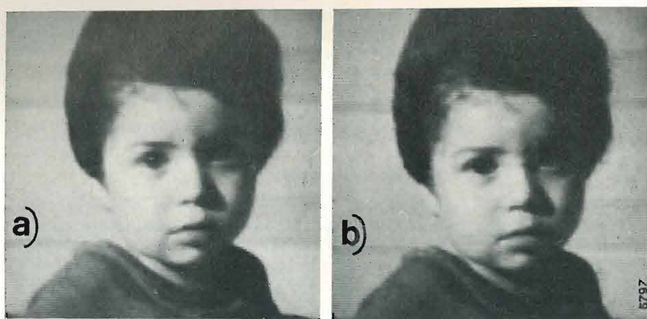
Fig. 7. — a), b): M = 16, \beta = 100, C.T. = 100\% ; — a): L = 32, \tau_c = 63,6\%, E.R.M. = 0,01249, E.Q.M. = 1,42684 ; — b): L = 16, \tau_c = 51,1\%, E.R.M. = 0,02196, E.Q.M. = 2,65098 .
