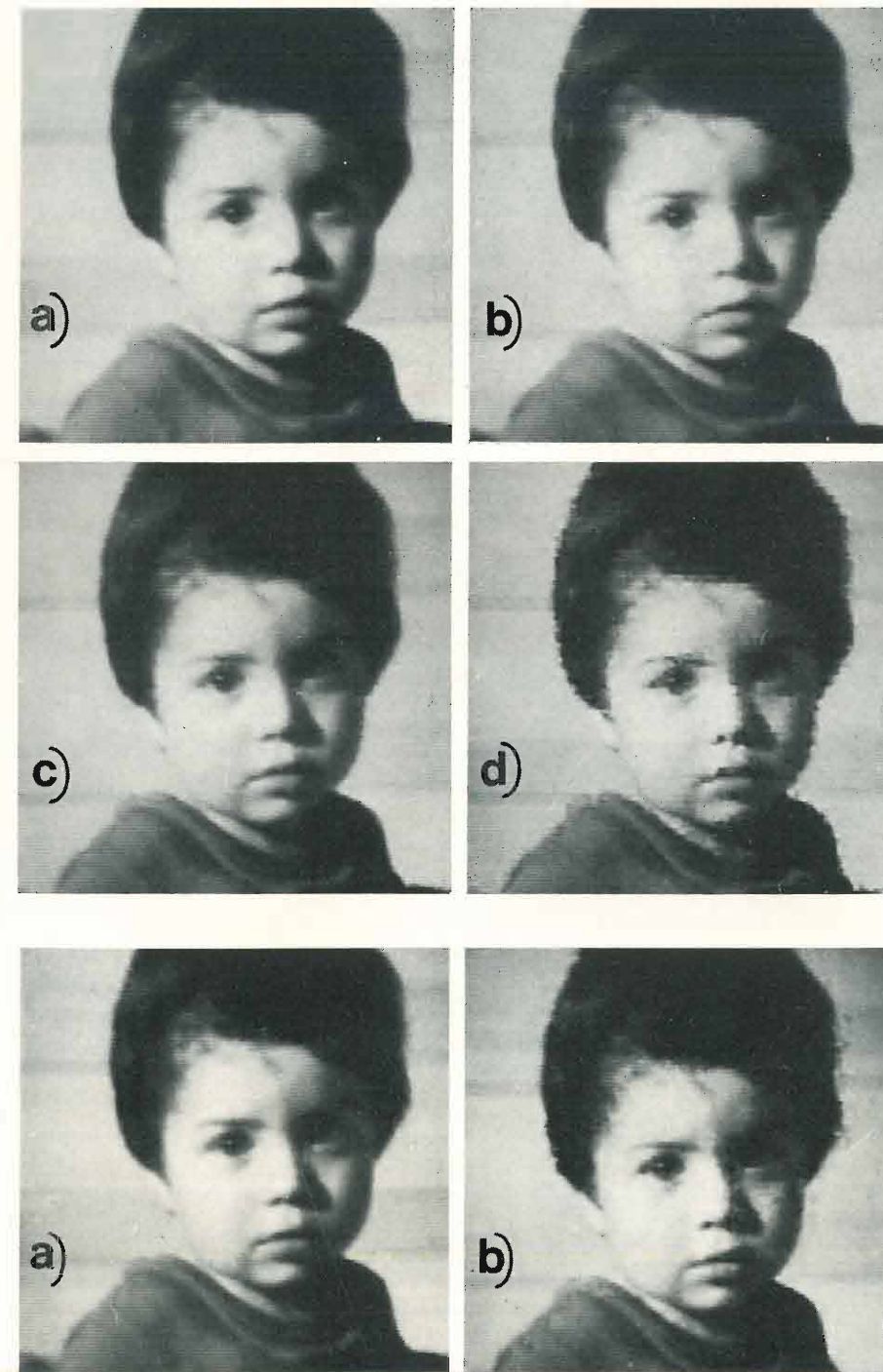
Fig. 5. — a) immagine originale: M = N = 128 , L = 256 , K = 8 ; — b), c), d): M = 4 , \beta = 100 , C.T. = 100 %; — b): L = 16 , \tau_c = 62,2\% , E.R.M. = 0,01021, E.Q.M. = 1,52577; — c): L = 8 , \tau_c = 50\% , E.R.M. = 0,01181, E.Q.M. = 1,75644; — d): L = 4 , \tau_c = 38,2\% , E.R.M. = 0,02982, E.Q.M. = 5,25765.
